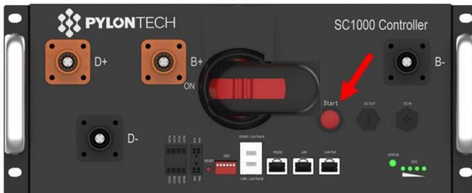
Figure 4-3: Front side of battery rack
